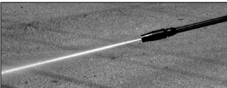
Figure 3 - Narrow high impact stream
