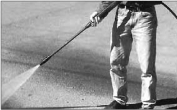
Figure 6 - Optimum Angle to Cleaning Surface.
