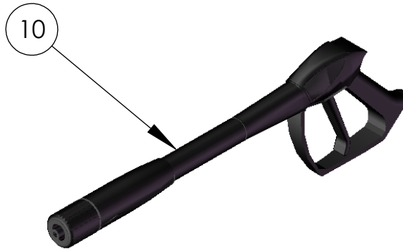
GUN & WAND 5075PSI, 3/8 PLUG X M22-F OUT (PART NO. 7103240)
