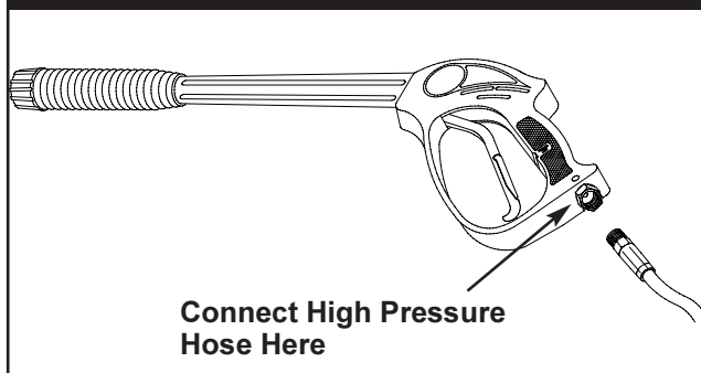
Figure 6 – Connect high pressure hose to spray gun.
