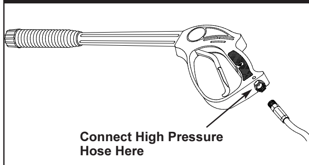
Figure 4 — Connect high pressure hose to spray gun.
