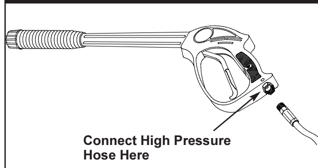
Figure 6 – Connect high pressure hose to spray gun.
