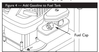
• Install fuel cap and wipe up any spilled gasoline.
