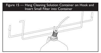
Place small filter of the detergent siphoning tube into the detergent container.
