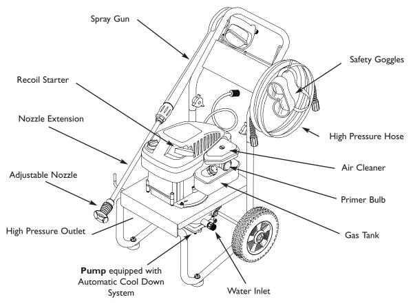
**Adjustable Nozzle** — Always attached to nozzle extension. Adjustable nozzle allows you to adjust pressure of spray and spray pattern.
