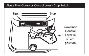
**NOTE:** For a warm engine, be sure the governor control lever is in the "**Fast**" position.
