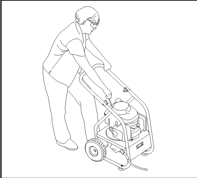
Figure 15 — Recommended Engine Starting Posture
