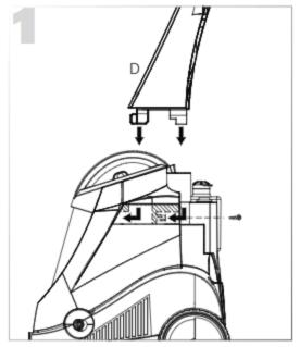
Connect the up-handle assembly (D) to the main unit and secure it by tightening the screws.
