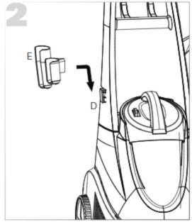
Attach the gun holster (E) to the up-handle assembly (D).
