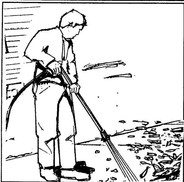
Figure 17 — Testing the Spray Pattern
