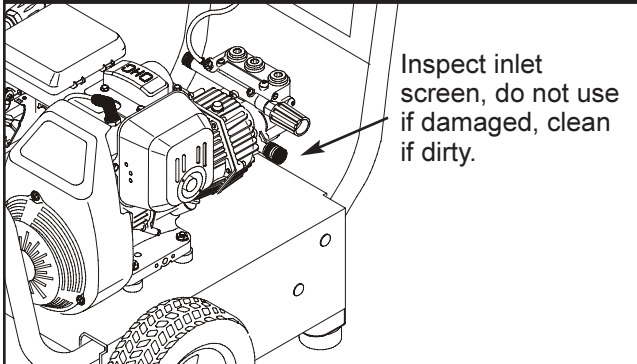
Figure 6 — Connect the Garden Hose to Water Inlet and Turn ON the Water.
