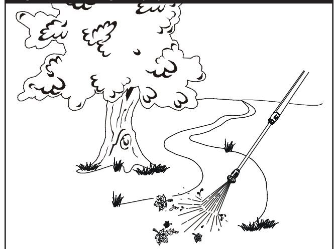
Figure 10 — Testing the Spray Pattern
