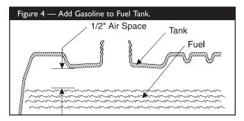
• Install the fuel cap and wipe up any spilled gasoline.
