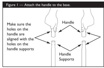
**NOTE:** It may be necessary to move the handle supports from side to side in order to align the handle so it will slide over the handle supports.
