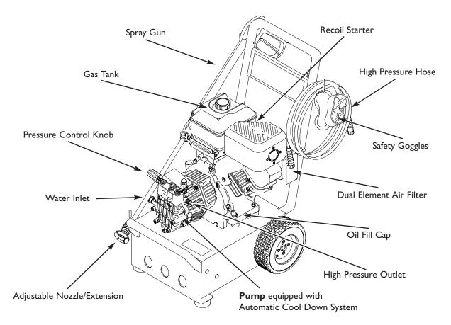
**Adjustable Nozzle/Extension** — Always attached to nozzle extension. Pull back for high pressure or push forward for low pressure; turn clockwise for narrow spray or turn counterclockwise for fan spray.
