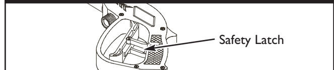
Figure 10 — Spray Gun with Safety Latch Engaged
