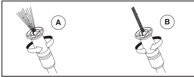
Figure 15: Adjusting the nozzle for spray pattern
