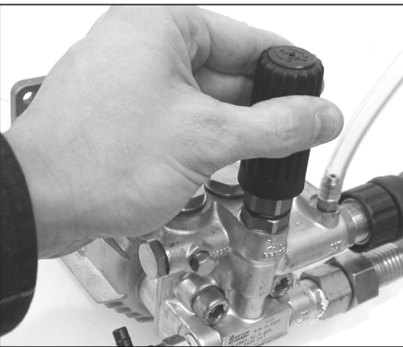
Figure 13 - Axial pump pressure adjustment
