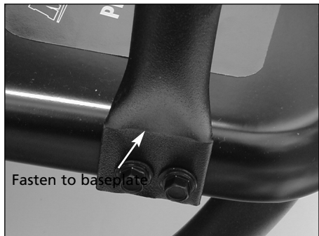
Figure 4 - Attach front guard tube (if applicable)
