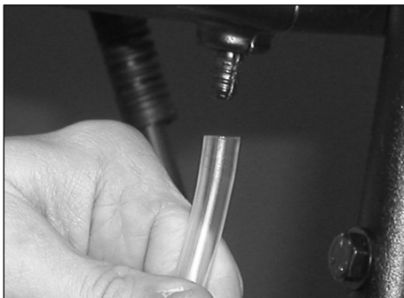
Figure 3 - Attach suction tube to barb fitting
