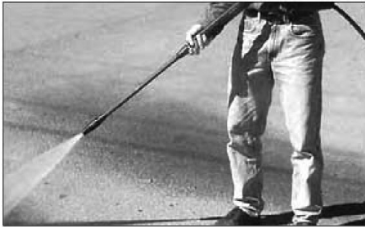
Figure 6 - Optimum Angle to Cleaning Surface.
