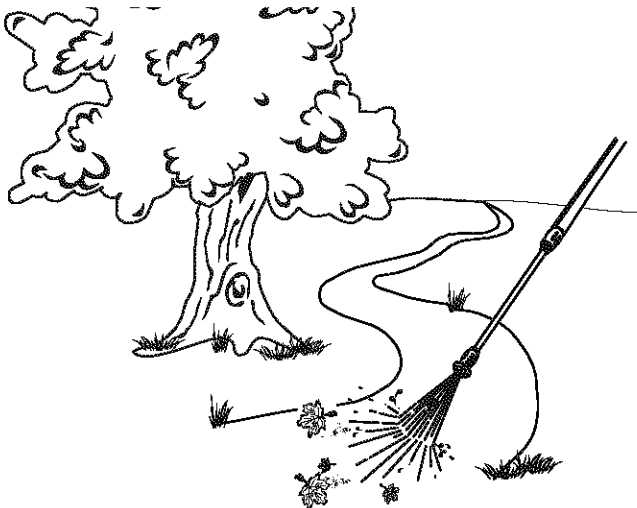
Slide nozzle forward for low pressure mode and detergent application.
