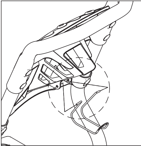
Figure 3 – Install Hose Hook
