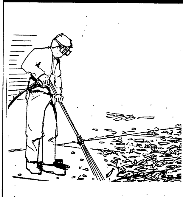
FIGURE 13 — Testing the spray pattern.
