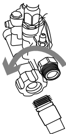
Figure 2-9. Connect Water Supply Hose
