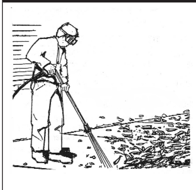
Figure 12 – Testing the Spray Pattern.
