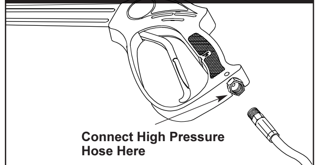
Figure 6 — Connect high pressure hose to spray gun.
