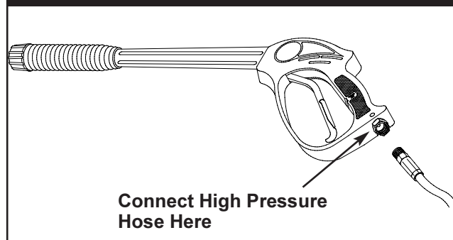
Figure 6 — Connect high pressure hose to spray gun.
