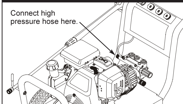
Figure 5 — Connect High Pressure Hose to Pump
