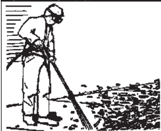
Figure 14— Testing the spray pattern.
