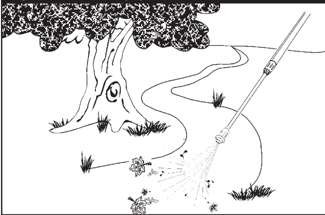
Figure 15 — Test the Spray Pattern.
