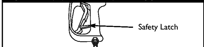
Figure 13 — Spray Gun with Safety Latch Engaged
