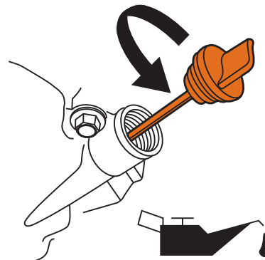
Figure 31 – Fill Engine Oil
