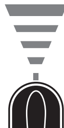
Low pressure fan jet for detergent injection
