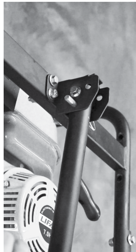
Locked in down position
