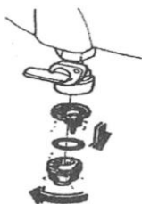
Fuel Filter Element Removal
