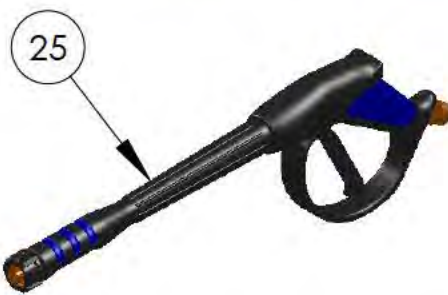
GUN, 3200PSI M22 MALE INLET X M22 F OUTLET (PART NO. 106725)
