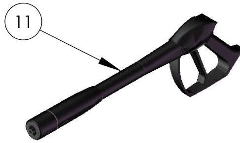
GUN, 5075psi 3/8 QC-M x M22-F OUT (PART NO. 7103240)
