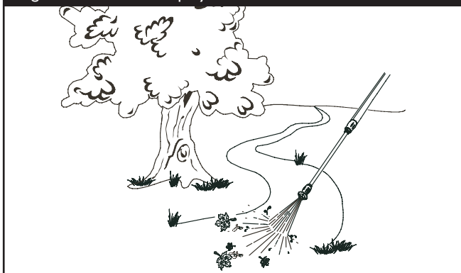
Figure 10 — Test the Spray Pattern
