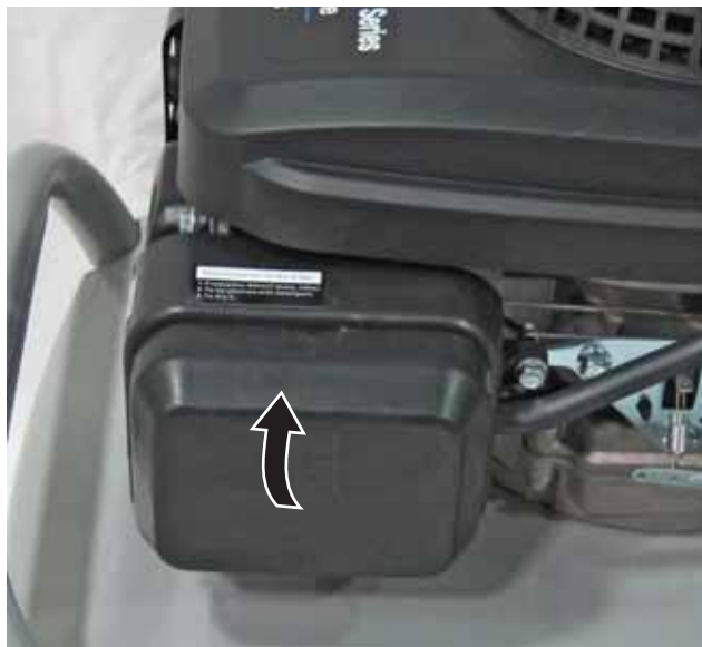
Figure 32 – Installation of Air Cleaner Cover
