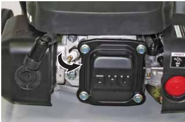
Figure 34 – Removing Spark Plug
