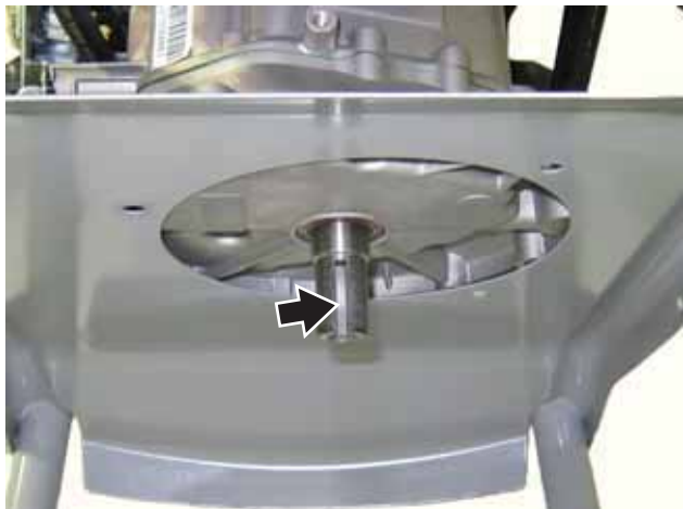
Figure 41 – Key and Crankshaft Keyway
