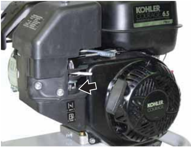
Figure 31 – Closing Fuel Shutoff Valve – WP3000
