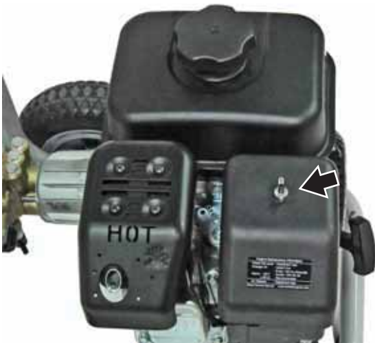
Figure 44 – Opening Air Cleaner Cover
